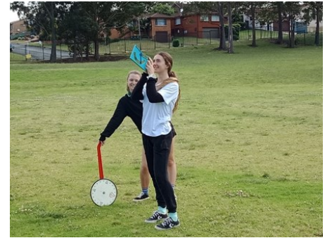
Karla C using the clinometer whilst Cerise M waits to measure the distance using the trundle wheel
